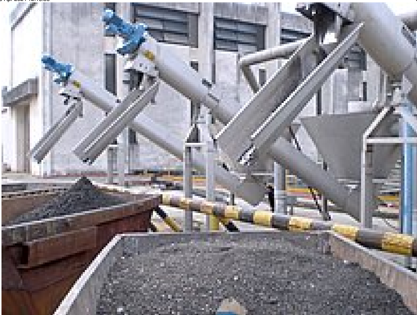
HUBER Grit Treatment System RoSF5: A universally usable and economical process of grit preparation solves your problems!
