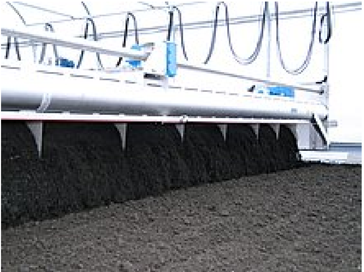
HUBER SRT system with HUBER Sludge Turner SOLSTICE®
