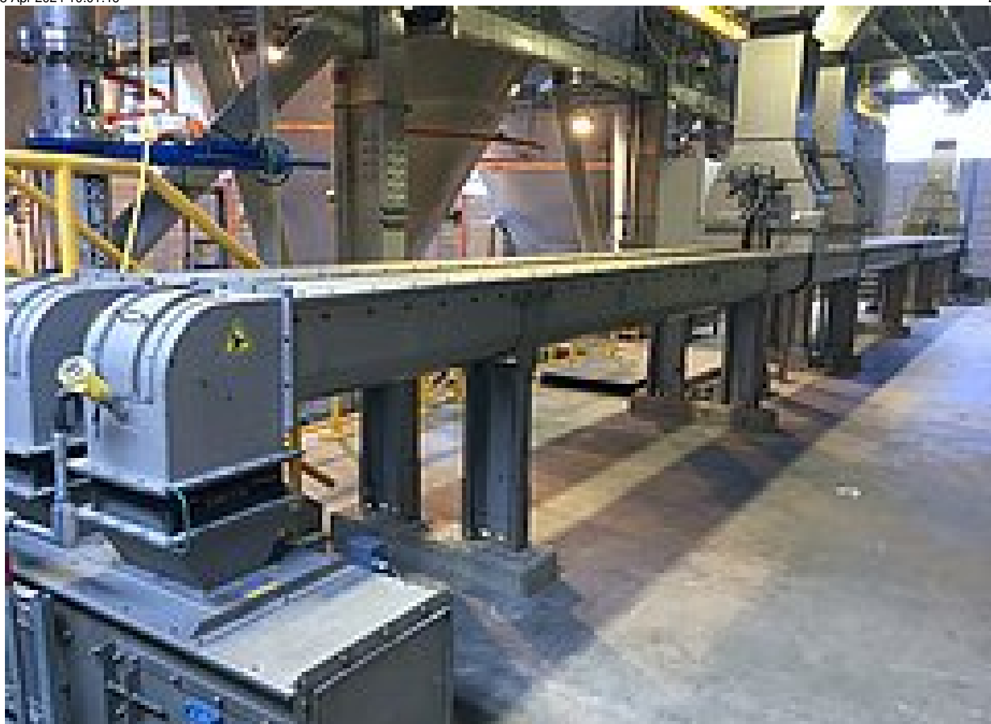
HUBER conveyor technology for sludge transport
