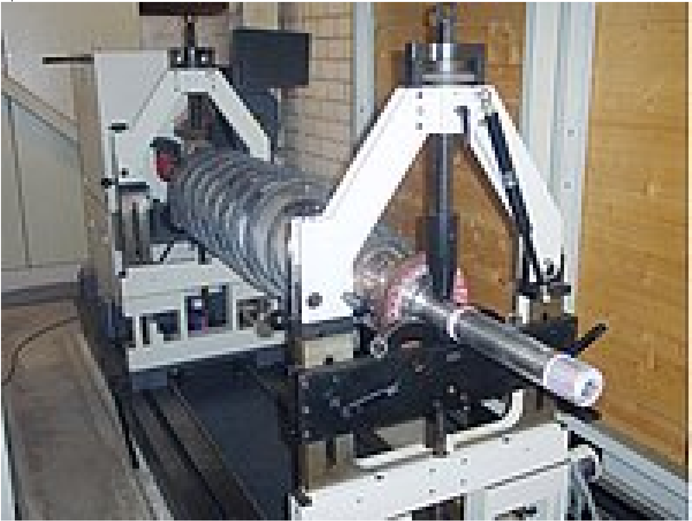
Centrifuge rotor on the balancing stand
