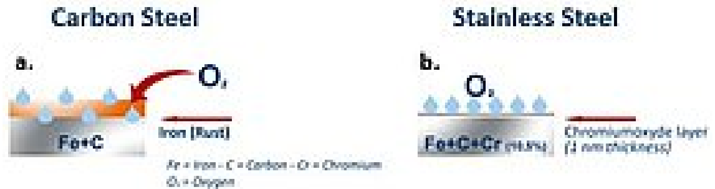
Figure 1. An illustration of the effect of oxygen on carbon steel and stainless steel
