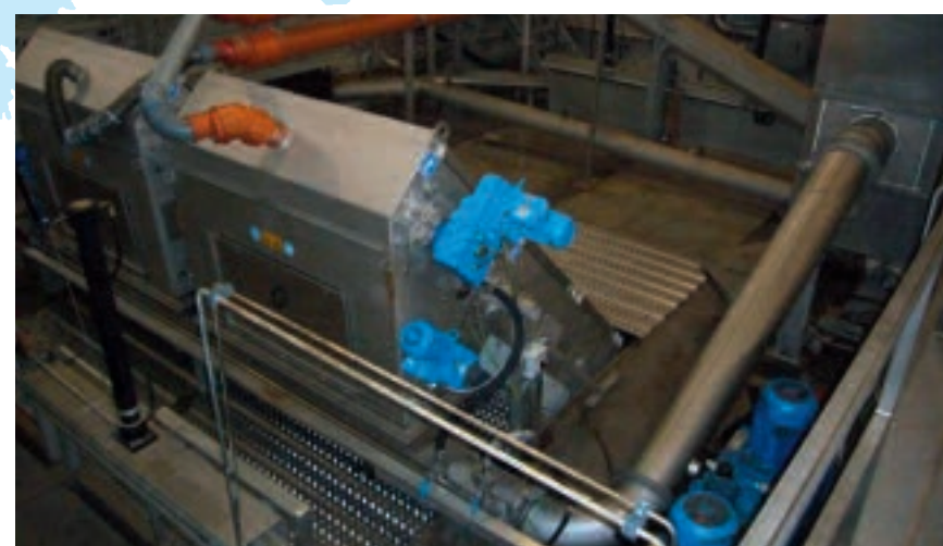
WAP with extra long feed trough up to 4,200 mm maximum has proven well for size 4 with standard guarantee values
