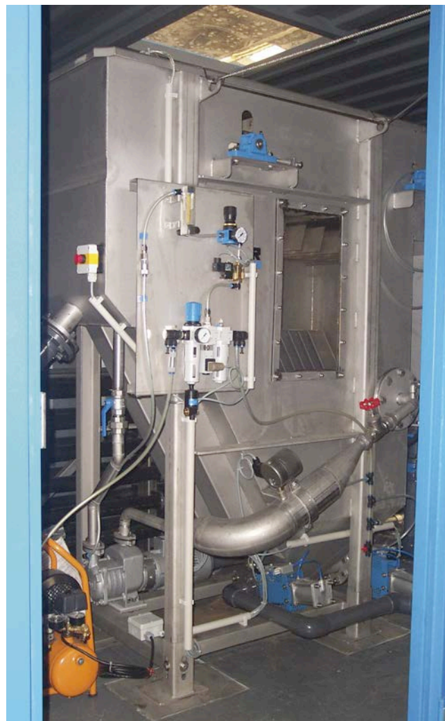
Dissolved Air Flotation test plant
