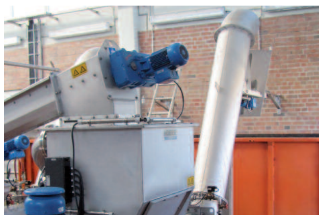
HUBER ROTAMAT® Screw Conveyor Ro 8t discharging screenings into a HUBER Wash Press WAP/SL
