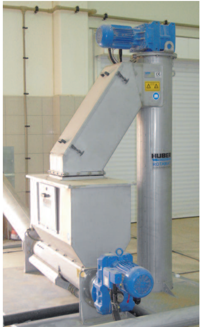
Vertical installation of a screw conveyor discharging screenings into a HUBER Wash Press
