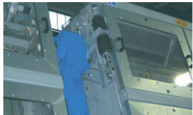
A torque restrictor reliably protects the screen against damage. The screen's controls combine reliability with adjustability.
