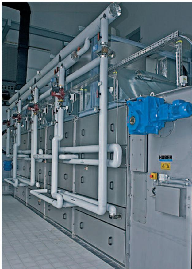
*Biogas exhaust heat supply to a belt dryer*
