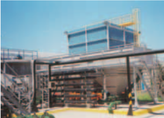
PEPSICO / Argentina: food processing, ROTAMAT® Micro Strainer Ro 9, HUBER Dissolved Air Flotation Plant HDF-75 with chemical treatment, throughput: 310 to 350 GPM (70-80 m³/h)
