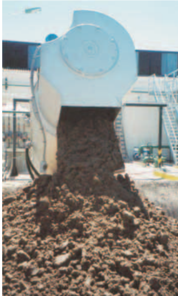
PEPSICO / Argentina: food processing, ROTAMAT® Screw Press RoS 3; Sludge cake with 25 - 30 % solids
