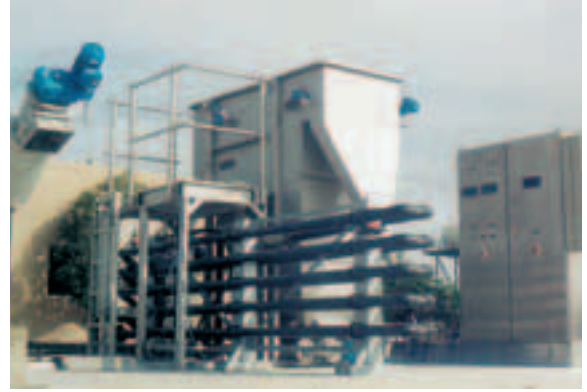
Slaughterhouse Medinat Zaved, U.A.E., ROTAMAT® Micro Strainer Ro9, HUBER Dissolved Air Flotation Plant HDF-1, throughput: 44 GPM (10 m 3 /h)
