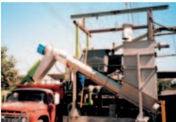
Slaughterhouse Carnes Darc / Chile ROTAMAT® Paunch Manure Press Ro7a, throughput: manure from up to 90 cattle per hour
