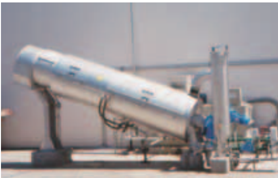
PEPSICO / Argentina: food processing, ROTAMAT® Screw Press RoS 3, Throughput: 22 to 44 GPM (5 - 10 m³/h)
