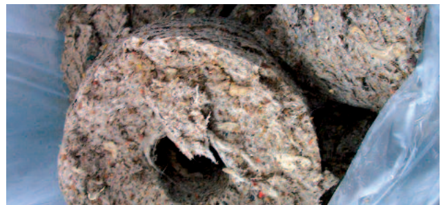
Washed and compacted screenings – the ideal fuel
