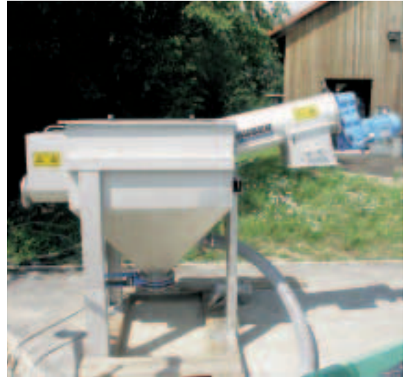
MiniCop screen and grit trap for pre-treatment
