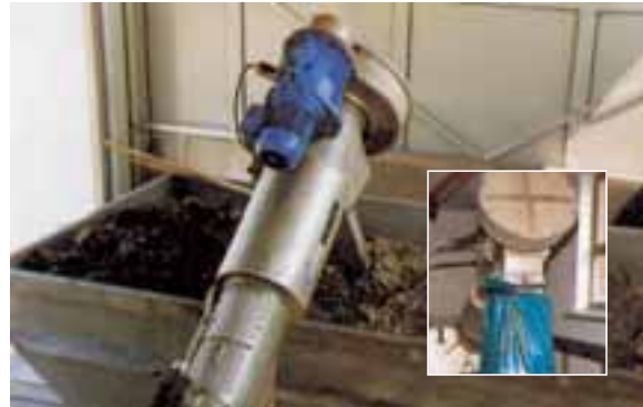
The dewatered screenings are discharged into a container or bag.
