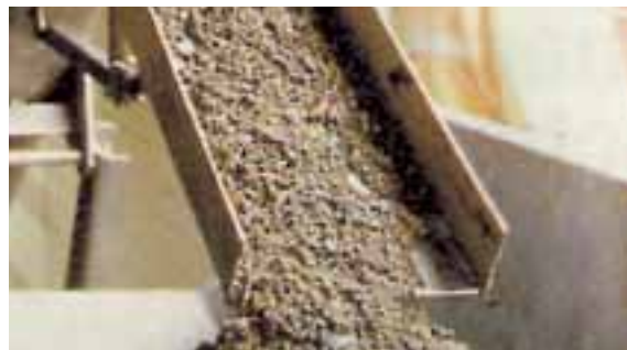
Discharge of grit
