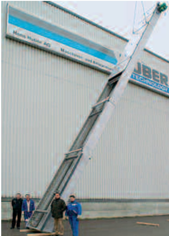
60 ft long and 6 ft wide RakeMax after successful factory testing
