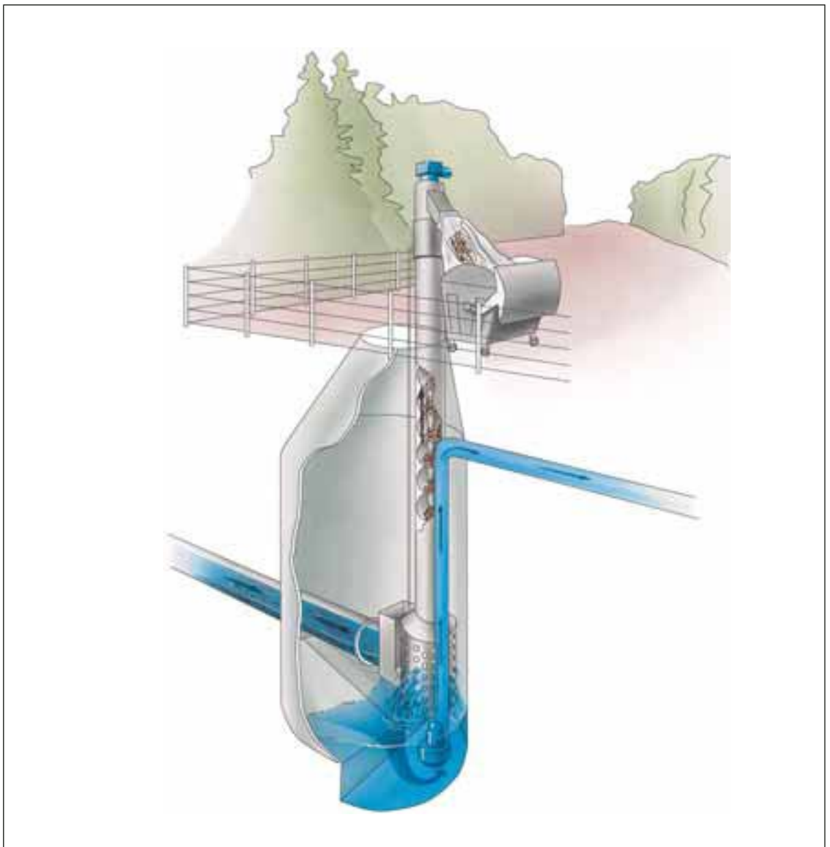
RoK 4 screen installation in a confined pump station
