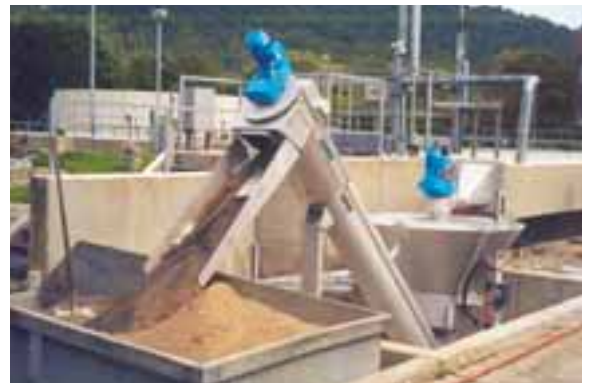
Grit Washer RoSF 4 Reduces the organic content in the grit to below 3%.
