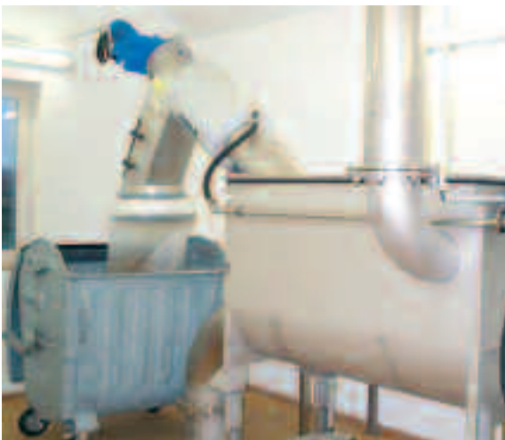
Tank-mounted ROTAMAT® Rotary Drum Fine Screen Ro 2 ...
